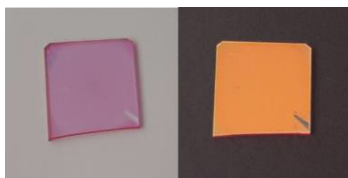
Figure 1.- Picture of a J-aggregate thin film deposited on top of a glass and located on top of a white (left) and black (right) paper. The reflected color shows a strong metal-like band in the orange.
